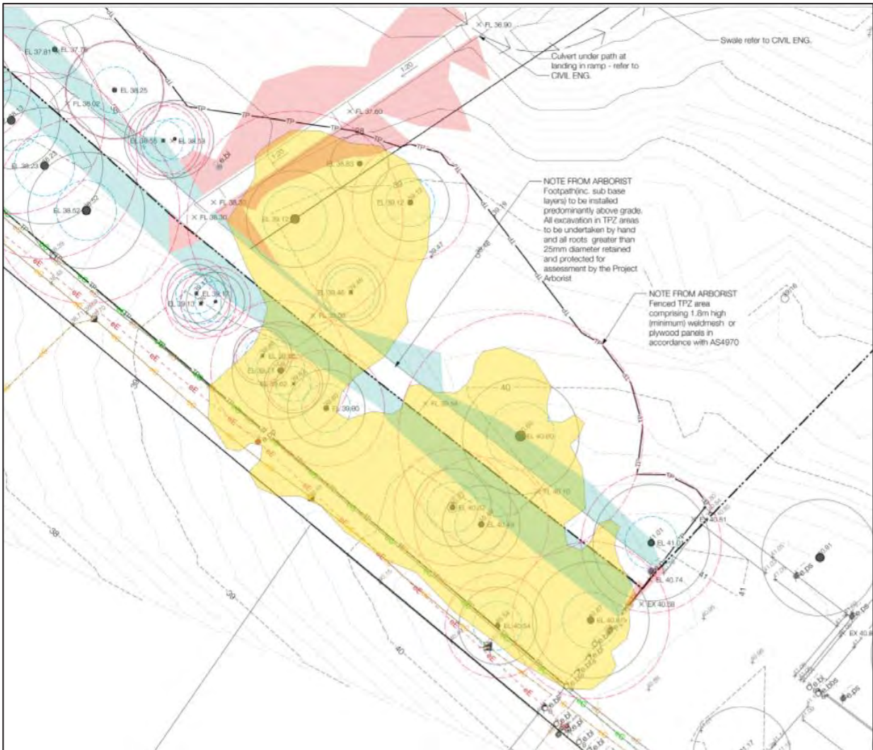
Figure 2: Area mapped under the Biodiversity Values Map (BVM) (shown in yellow) and proposed pathway demonstrating that all trees within the BVM can be retained (McGregor Coxall 2020)
